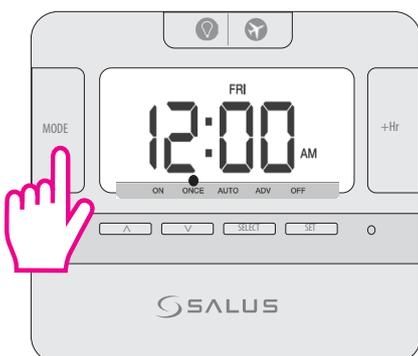
Pressing the Mode key twice activate the ONCE Mode. In ONCE mode, the controller gives the boiler the command to run only for one period per day (from program 1 ON to program 3 OFF)
