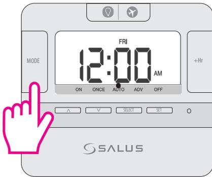
Pressing the Mode key 3 times activates the AUTO. In AUTO mode, the controller gives the boiler the ON/OFF command depending on your schedule.
