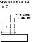
5 = orange Connection of external switching contact
