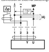
A) additional MP-Bus nodes (max. 8) • Switching current 16 mA @ 24 V
