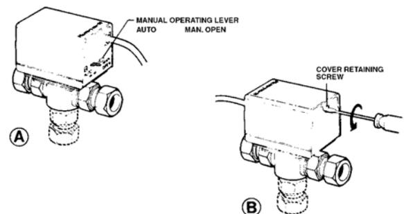
Fig. 1. Removing Cover
