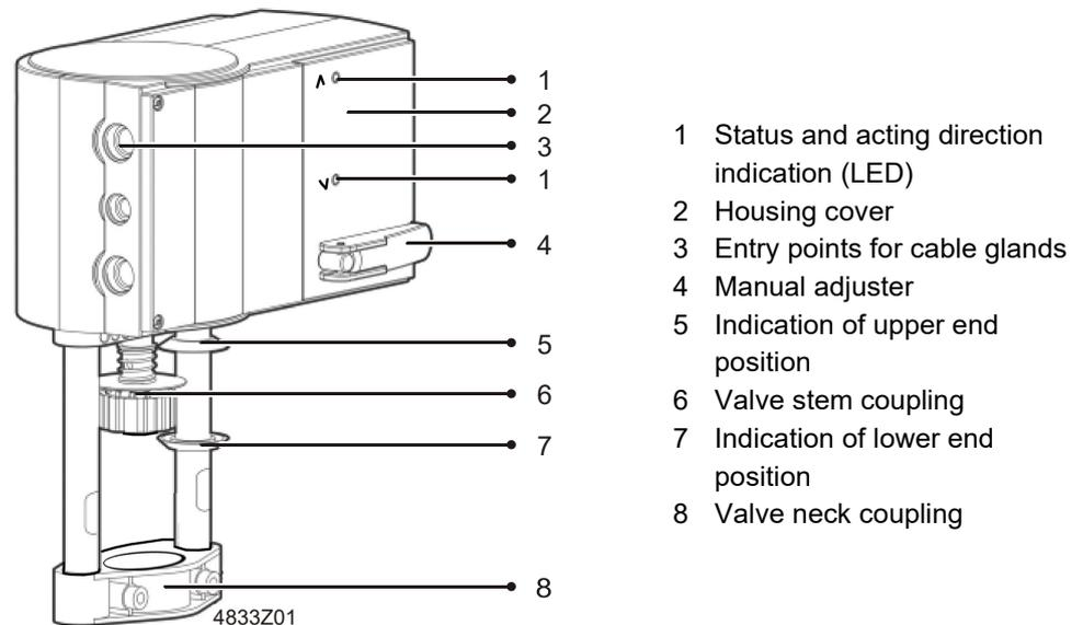
The actuator can be operated as a 3-position or modulating actuator in two acting directions depending on the type of connection. It is suitable for both PICVs VPF.. with 20 mm stroke as well as for valves with a 40 mm and 43 mm stroke. The stroke is calibrated automatically during initialization.
