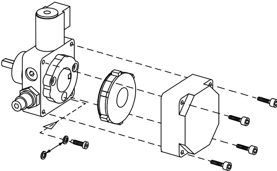
In case of one-pipe operation the horse-shoe-shaped washer will be mounted under the screw head, and in case of two-pipe operation, the horse-shoe-shaped washer will be removed.
